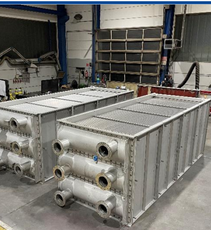
Heat exchanger in production
